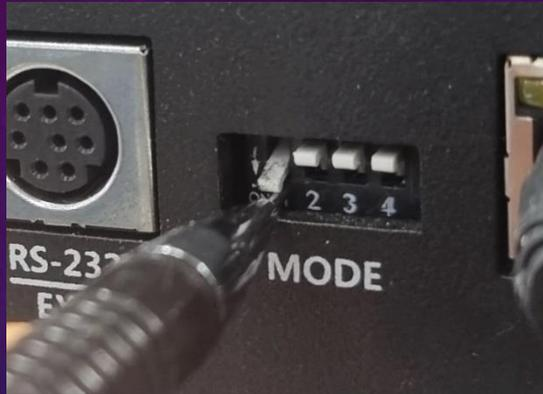
Set proSTICK to firmware update mode by turning down DIP switch . Then, turn the power off and on again.
